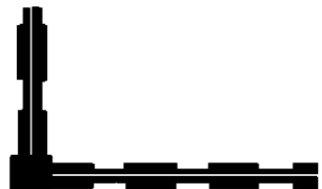
ALTERNATE BOARD Boards are in the same position on opposite sides of the stringer
